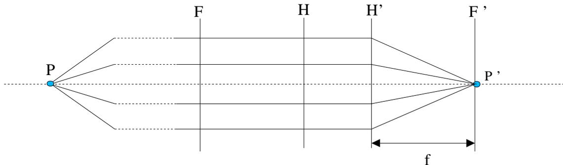
If you assume that P is indefinitely far away, all beams of light are parallel and focused in the focal layer in P'. So the distance between the main layer and the film should be the focal distance (200 mm), to get a sharp image.
