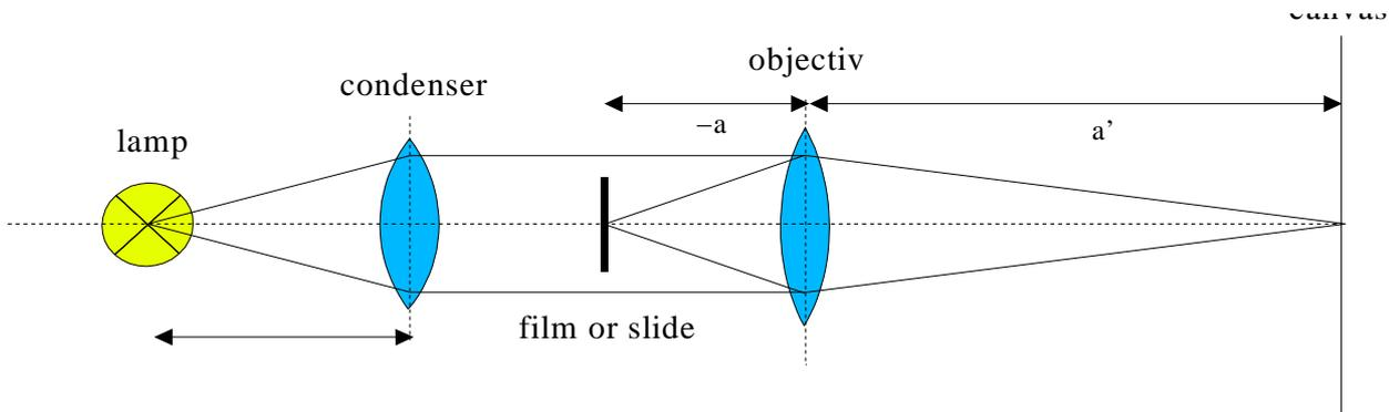
The lamp should be in the absolute focus of the condenser lens to get parallel beams on the other side. For a and a' the following equation applies:
