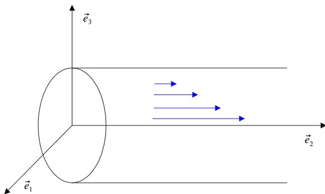
$$\vec{v}(\vec{x}) = \vec{v}(x_1, x_2, x_3) = c \begin{pmatrix} 0 \\ R^2 - x_1^2 - x_3^2 \\ 0 \end{pmatrix}$$
